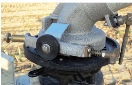
Figure 1. Device regulating rotation speed of the travelling gun
